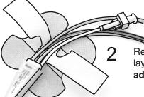
Remove cover from Velcro strip, lay "tubes" / lines into the adhesive area.
